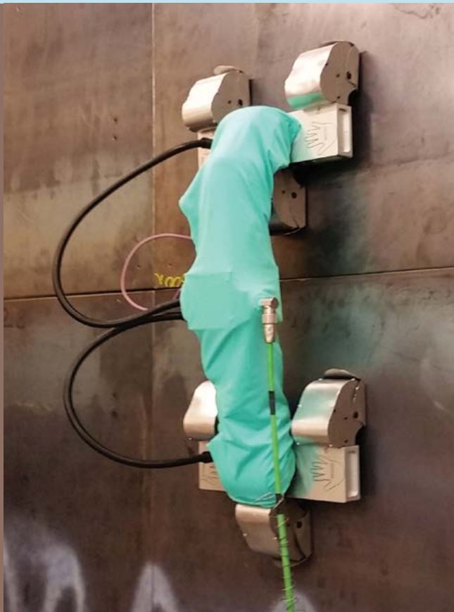
Autonomous climbing robot for inspection and condition assessment of confined spaces. Credit: University of Technology Sydney.
